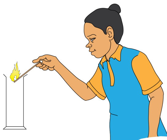
Fig 6.6: Testing for collected gas
