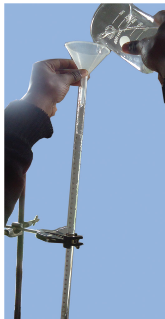
Fig 7.6: Correct method of filling a burette
