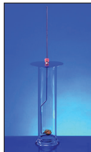
Fig 1.9 Burning charcoal in oxygen
